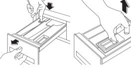
tap. To remove the drawer from the machine, press the button in the rear left-hand corner.
